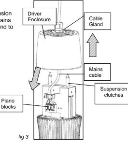
3. Wire the cable in as shown in fig 4 to the piano blocks, the maximum recommended cable cross sectional diameter is 1.5mm.
