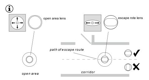
For best photometric performance ensure that the long axis of the escape route lens in line (parallel) with the line moulded in the cover plate. These lines should then be positioned along the path of the escape route as shown above.
