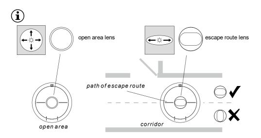
For best photometric performance ensure that the long axis of the escape route lens in line (parallel) with the line moulded in the cover plate. These lines should then be positioned along the path of the escape route as shown above.
