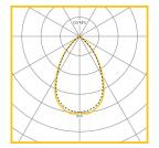
Narrow beam, semi specular LOR = 100% SHR MAX = 0.71 Medium beam, semi specular LOR = 100% SHR MAX = 1.25
