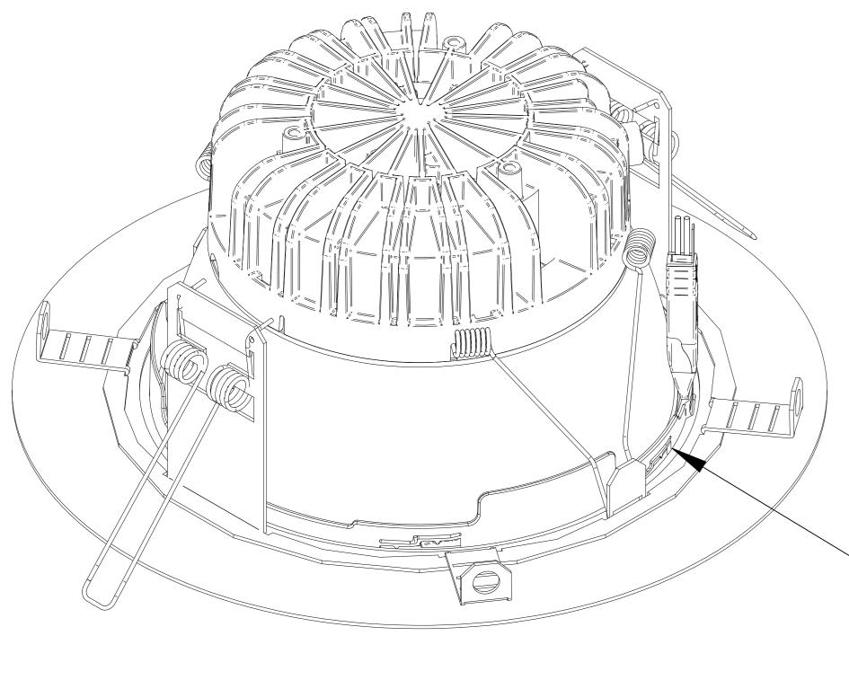
Step 2 - Install the fitting by bending up the springs 90 degrees then insterting them into the retro fit bezel aperture. Then releaseing the product so that it pulls up flush to the retro fit bezel front surface. Ensure that the gasket on the product seal all the way around the aperture.
