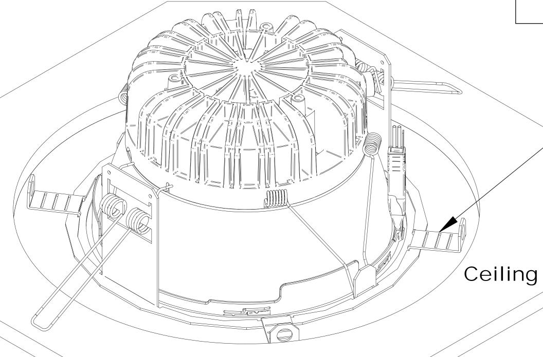
Step 3 - Fold 4 tabs as shown to centre the bezel in the hole there are a number of different easy folds for different diameters select bend closest to your hole size
