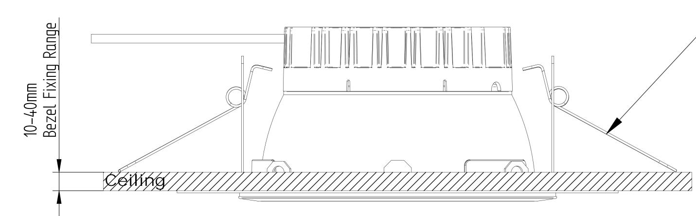
Step 6 - Fold back the springs on the retro fit bezel and place them through the ceilig void and release so that the bezel is held up against the ceiling
