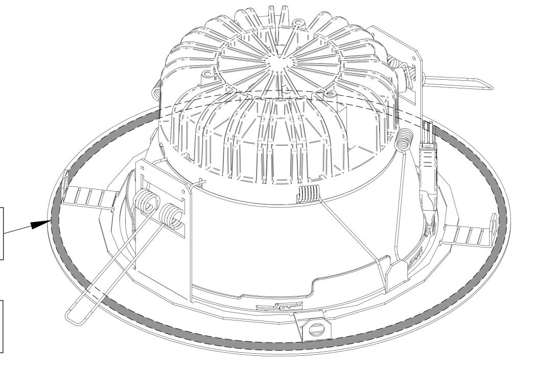
Step 4 - Apply mastic around the circumference of the bezel in one continous loop to make a seal to the ceiling
