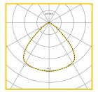
Medium beam, semi specular LOR = 100% SHR MAX = 1.13 Wide beam, semi specular LOR = 100% SHR MAX = 1.69
