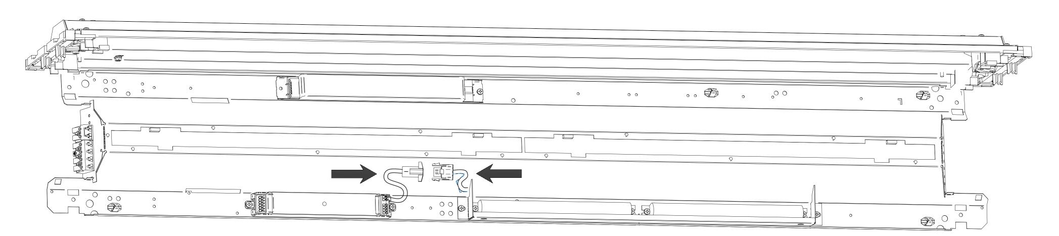
c) Refit the geartray assembly to the horizontal position ensuring that the clips are fully engaged at both ends.
