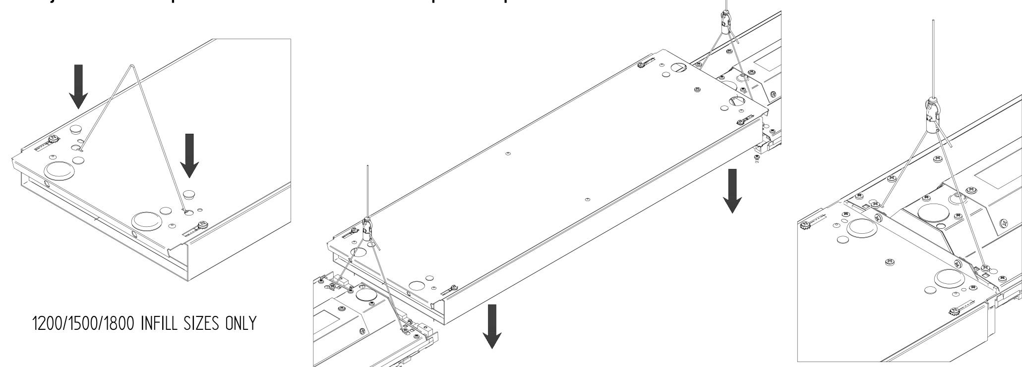
c)Fit the supplied jointing screws into the adjacent luminaires, but do not fully tighten at this stage.
