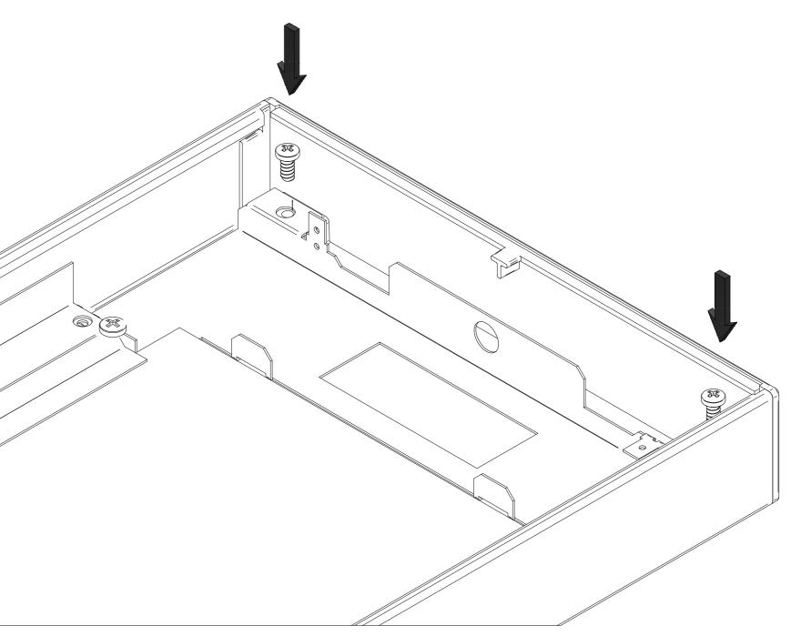
10a. Re-attach earth & safety cords to the diffuser assembly & connect Sensor plug where fitted. 10b. Align the front diffuser assembly with the canopy & re-attach to canopy by pushing up from the front until hook on both sides are fully clipped over the canopy edge along the entire length. Nb Care should be taken to ensure that no cables are trapped during the fitting process.
