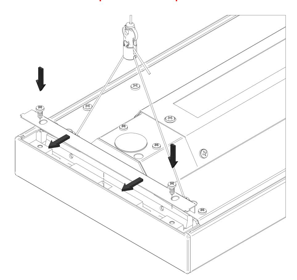
Nb - LOOP SECONDARY SUSPENSION - CABLE THROUGH SLOTS HERE WHEN NECESSARY.
