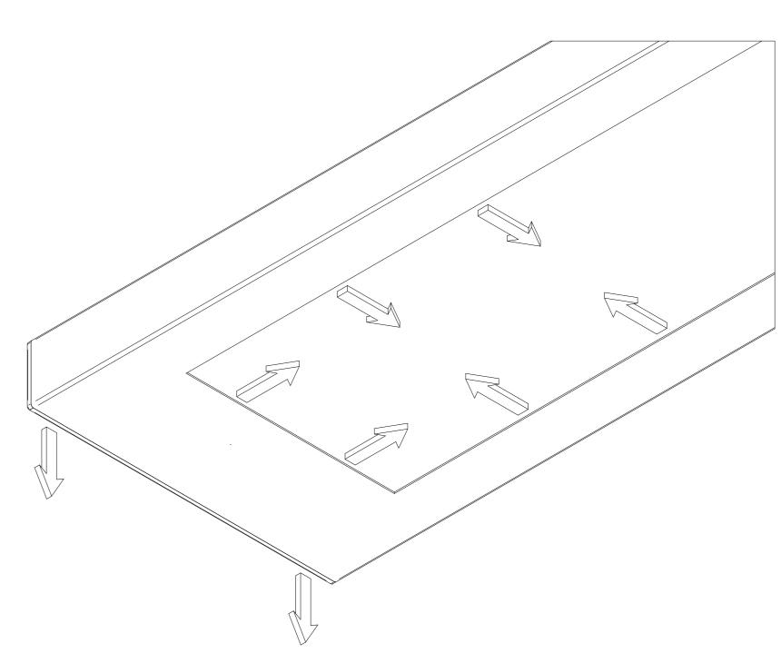
Drainage Path for any ingresss of water via diffuser & endcap joint as indicated above.
