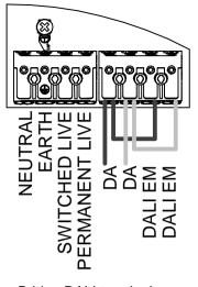
Bridge DALI terminals as shown if the driver and inverter share a single DALI pair. Use link wires supplied
