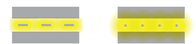
Linear solutions require fewer installed points to light the same space than point source solutions
