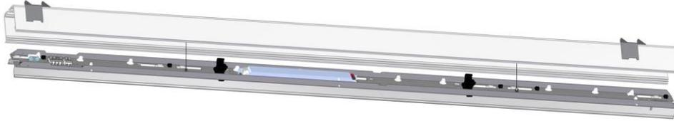
9. On continuous end of run fittings, endcaps will need to be installed. This can be done before the product is installed into the ceiling or whilst in the ceiling depending on space and scenario. Endcap fitting can only be achieved with the gear tray removed as per previous step.
