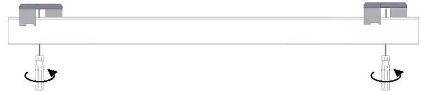
7. Depending on the scenario the mains cable can be fed from the back by piercing the rubber grommet. If no access to the back is available eg. In plaster board ceilings then the cable will need to be feed into the product before it is offered into the void.
