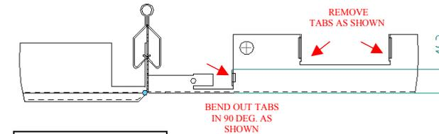
SAS international Omega bar 154 system – Remove tabs as shown, bend out corner tab at a 90 degree angle and clip recessing panel into spring and pull front face of the luminaire up to the panel.
