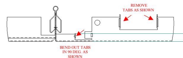
Burgess Architectural Ltd A bar spring tee system – Remove tabs as shown, bend out corner tab at a 90 degree angle and clip recessing panel into spring and pull front face of the luminaire up to the panel.
