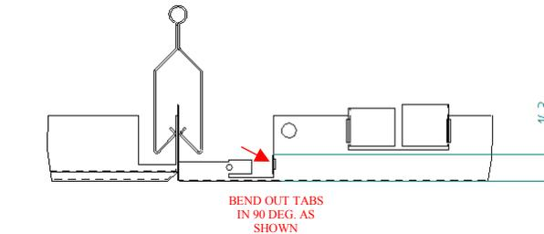
SAS international Omega bar 154-S system – bend out corner tab at a 90 degree angle and clip recessing panel into spring and pull front face of the luminaire up to the panel.
