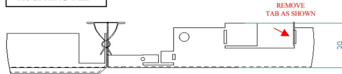
SAS international 120 spring tee bar system – Remove tabs as shown and clip recessing panel into spring and pull front face of the luminaire up to the panel.
