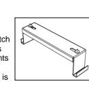
2. Mark suspension centres on ceiling and prepare the surface for mechanical fixings. Secure the ceiling attachments in position using a suitable screw or machine
