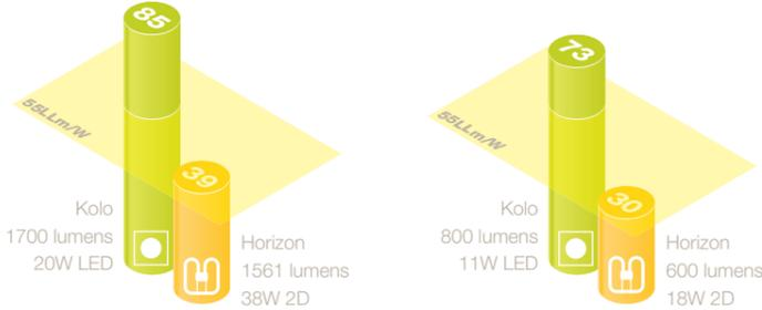
In a typical corridor application, Kolo uses only half the power of the equivalent fluorescent luminaire. As a direct replacement, this will yield an energy saving of over 50%. As an alternative, the higher power Kolo can be used to reduce the installed points and associated installation costs, whilst still delivering a similar energy reduction.
