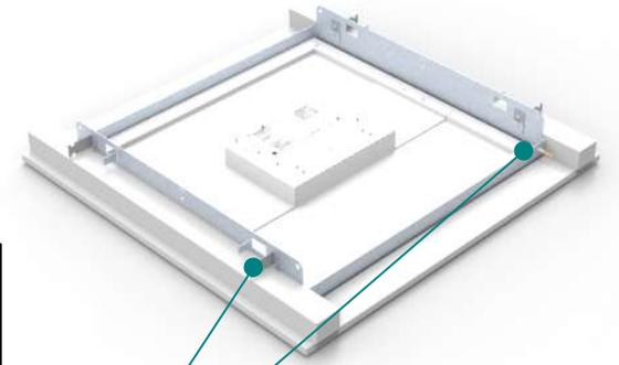
FOR SECONDARY FIXING POINTS THE CUT OUTS ON PLASTER BOARD FRAME CAN BE USED. ON THE LUMINAIRE FOLD UP CORNERS TO PROVIDE 4 FIXING POINT OPTIONS
