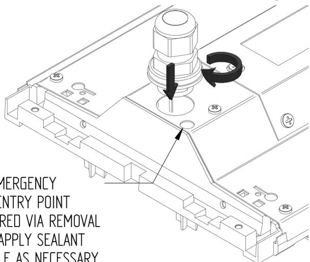
SEPARATE EMERGENCY DALI CABLE ENTRY POINT WHEN REQUIRED VIA REMOVAL OF PLUG. NB APPLY SEALANT AROUND CABLE AS NECESSARY
