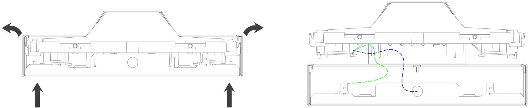
5a. Fit 'Y' splitter adjustable suspension hanger cables into the canopy keyhole cutouts and fit the included locking screws into the adjacent holes to secure.
