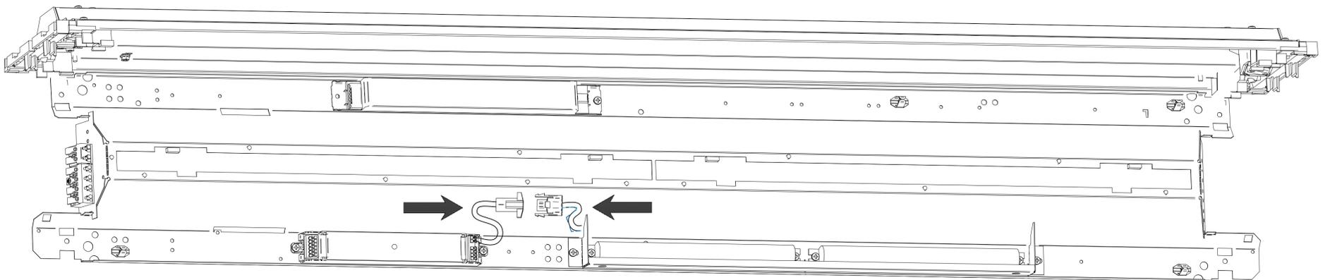
c) Refit the geartray assembly to the horizontal position ensuring that the clips are fully engaged at both ends.
