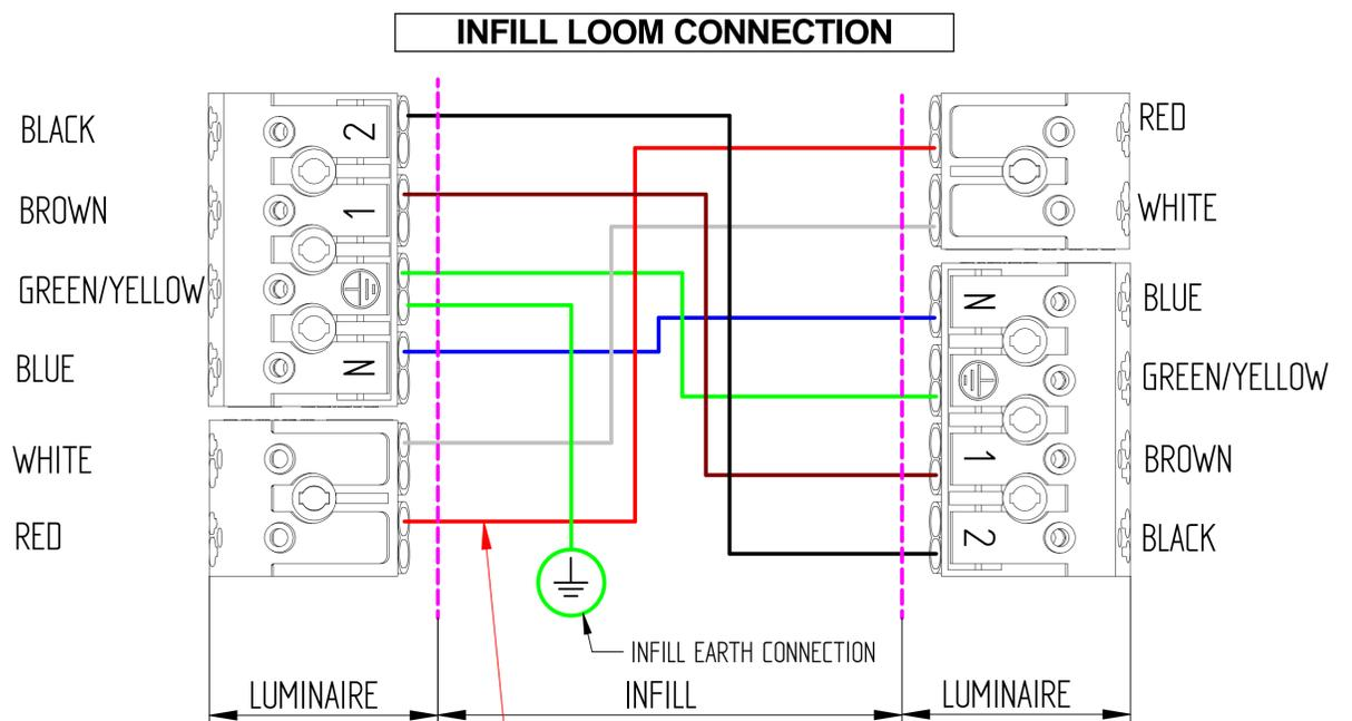
**NB - FOR OR3 COMEPS PORTAL CONFIGURATION REMOVE THE RED & WHITE CABLES FROM THE WIRING LOOM. ! DO NOT CONNECT TO THE DALI TERMINAL BLOCKS**
