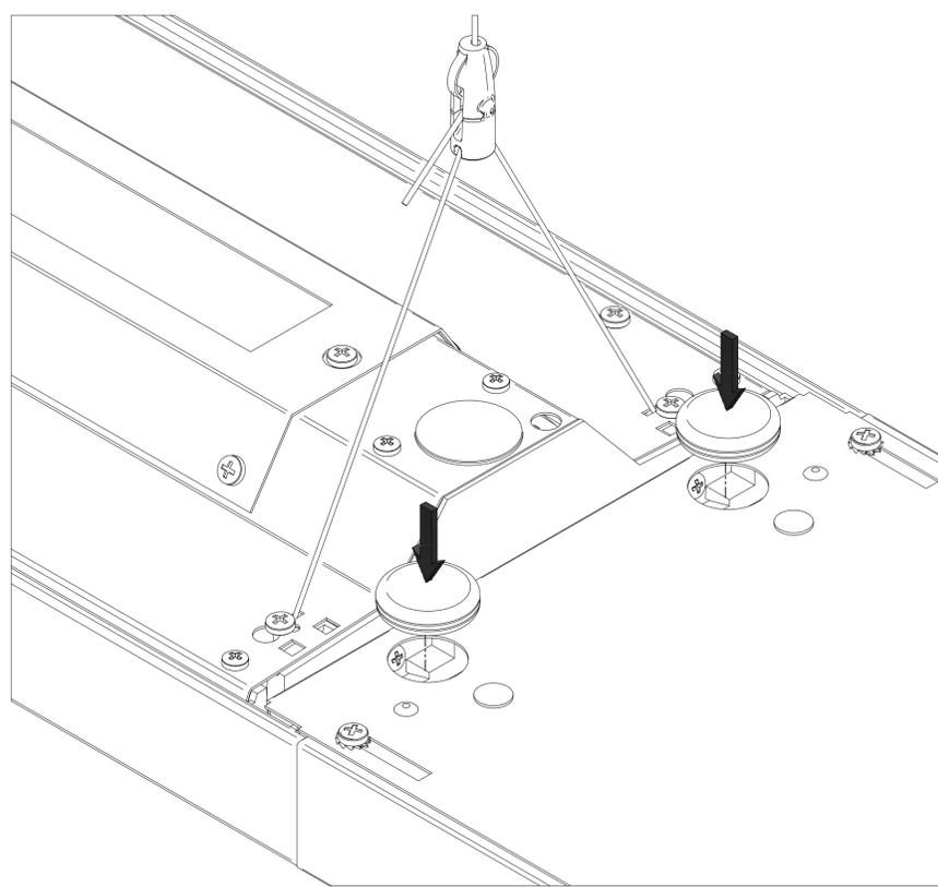
12. Fit locking plates at each end of continuous rows & individual luminaires with screws provided. Ensure that the plate overlaps the outer endcap at each end before fully tightening the screws.
