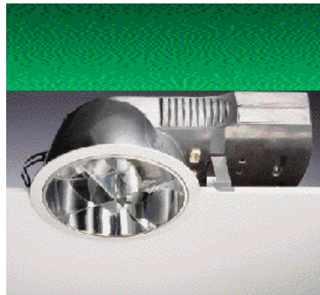
Due to its horizontal lampping and compact integrated housing, the depth of the Mirage MD20 is just 112mm. This allows it to be sited in ceiling voids otherwise considered too restrictive for fluorescent downlighters.
