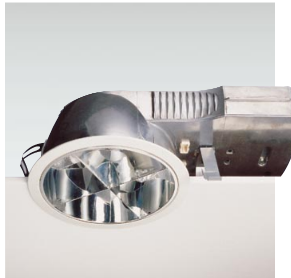
Due to its horizontal lamping and compact integrated housing, the depth of the Mirage MD20 is just 112mm. This allows it to be sited in ceiling voids otherwise considered too restrictive for fluorescent downlighters.
