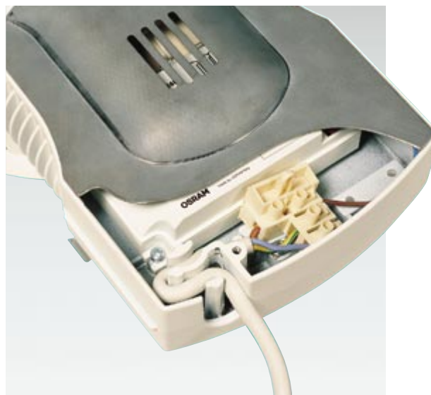
Top section showing tilted terminal block and labyrinth cable strain relief to ease installation.
