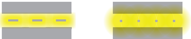
Linear solutions require fewer installed points to light the same space
