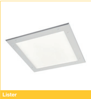
Lister IP65 rated where treatment demands a higher level of infection control. Incorporating Nhex prism diffusing technology for areas of VDT use and to minimise discomfort glare to patient and practitioner.
