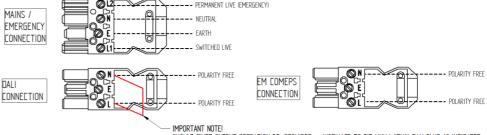
SHOULD FIXED OUTPUT OPERATION BE REQUIRED - INSTALLER TO FIT LINK WITHIN DALI PLUG AS INDICATED
