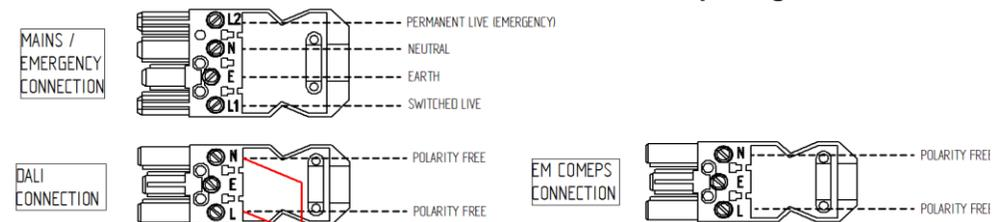
Nb - This Dali connection plug is not required on COM9 variants
