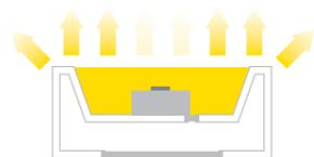
Epi Up LEDs use a bonding wire, which is prone to manufacturing issues and environmental contaminants
