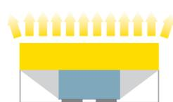
The e-light LED has a highly reflective base and unique architecture to further increase direct light output and drive even higher efficacy.
