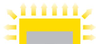
First generation Flip Chips typically have reduced package sizes but increased angle in direction of light resulting in poor light extraction
