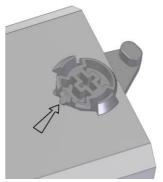
Make sure the pip on the cam bracket is aligned with the dimple in the round cutout as shown left.
