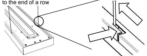
5. Pull suspension cables through the suspension cap to adjust the height of the Broadsword. Ensure the luminaire sits level. Maximum cable drop is 1.5m
