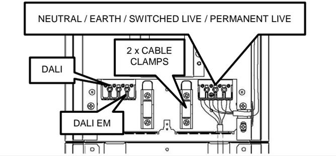
**9.** If setting up a continuous Broadsword review the wiring set up below. The mains cable enters the first Broadsword (step 7) and a link cable (supplied by others) connects from the first terminal block to the next luminaire. Cables are routed between the terminal blocks along the wire way. Note the exit and entry points shown below.
