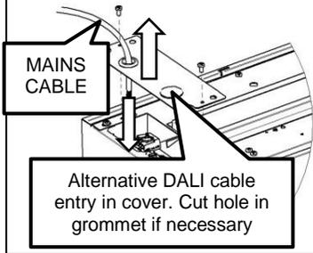
**8.** Terminal block wiring: Wire into the terminal blocks as shown below using the cable clamp to fix mains cable. Depending on the model the terminal blocks may differ.
