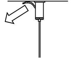
6. If installing a Standalone Broadsword luminaire skip to step 7. If setting up a continuous Broadsword remove the infill lids and attach onto the ends of the luminaire as shown using the bolts and washers supplied with the infill. These will align with the threaded inserts in the Broadsword continuous body. Make final adjustment to the suspension cables if required and snip off excess only when satisfied with height and level.
