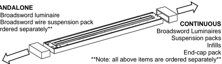
2. Mark out suspension centres in ceiling as shown below. Refer to dimensions table for drill hole centres. Ensure structure and fixings (supplied by others) are suitable to support the weight of the luminaire.
