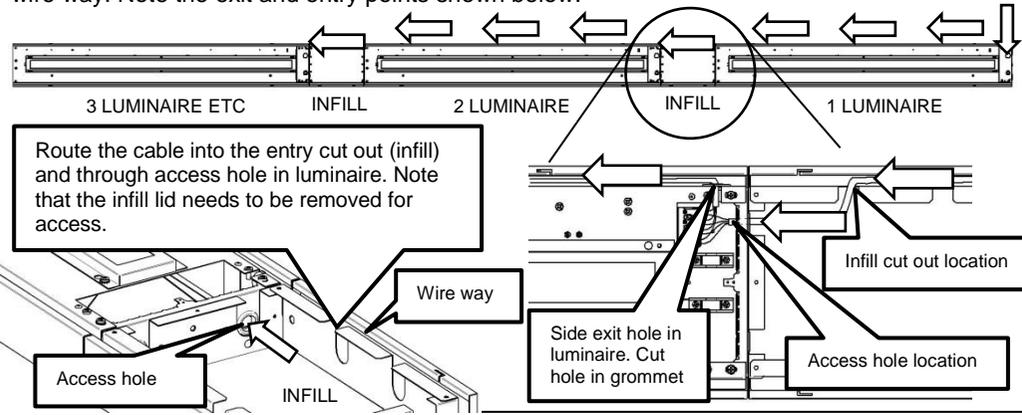
**10.** At the end of a continuous run of luminaires remove end grommets from the luminaire and attached ends caps as shown. Use screws provided. Re-attach infill lids.
