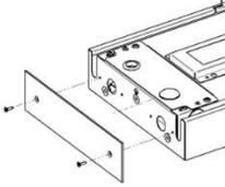
**11.** If the Broadsword has emergency / Comeps remove battery cover on the back of the luminaire and connect battery cables. See step 2 for cover location. Note the warnings on back of product!
