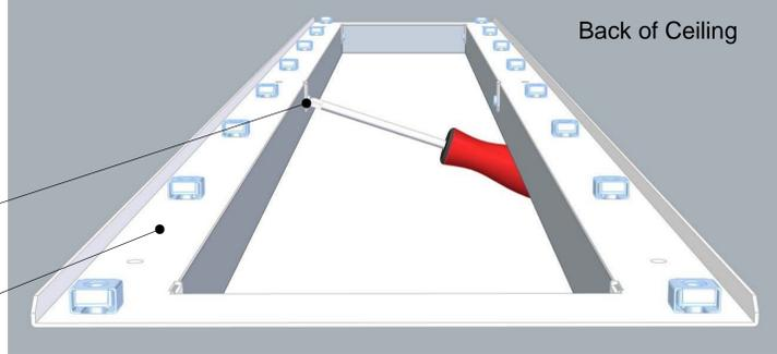
Step 3 - Lift and tilt the ceiling bracket into the ceiling void and place nutserts up as shown. Bend down the holding tabs on the edges of the aperture, align holes drilled in step 2 with ceiling bracket cagenuts. (Diffuser screws can be used to aid alignment but will have to be removed before cover installation) Then screw the ceiling bracket to the ceiling aperture edge using the 6x sidescrews supplied to secure the ceiling bracket in place. Ensure screw heads are as flush as possible
