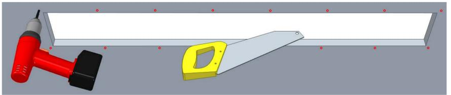
Step 2 - Drill the 16 marked holes with a 10mm drill bit. Ensure that the holes are drilled vertically as they need to align with the ceiling bracket nutserts.
