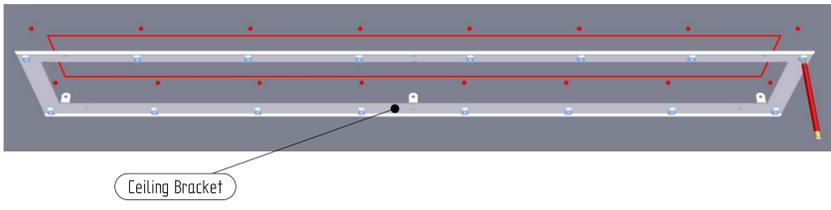
Step 1 - Hold the Ceiling Bracket up to the ceiling using screws to secure in place, in the required mounting position and mark out the inner aperture (1191mm x 140mm +3/-0) and 16 bezel holding holes through the nutserts. This installation is considered a two man operation.
