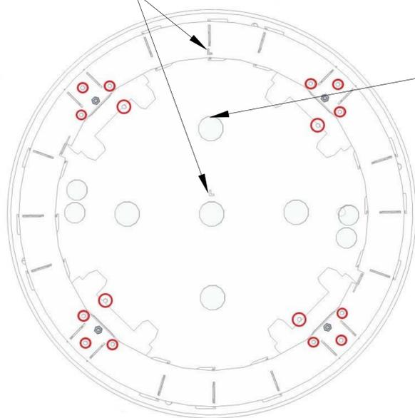
A temp. pilot screw can be fixed in place at the top of the hole indicated so the holes can be marked more easily.
