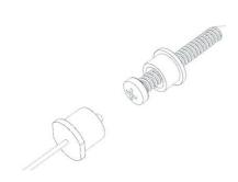
Screw the three flanged cups into the drilled holes in the ceiling. Thread a suspension cable through each of the round cups as shown and then screw the cups onto the fixed flange cups. Please use suitable ceiling fixings for suspending.
