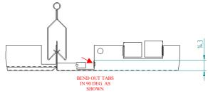
SAS international Omega bar 154-S system – bend out corner tab at a 90 degree angle and clip recessing panel into spring and pull front face of the luminaire up to the panel.
