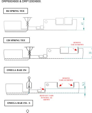
Burgess Architectural Ltd H4 spring tee bar system – Clip recessing panel into spring and pull front face of the luminaire up to the panel.
