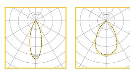
Narrow beam, semi specular LOR = 100% SHR MAX = 0.71 Medium beam, semi specular LOR = 100% SHR MAX = 1.25
