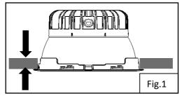
Check void dimensions. Ensure 100mm clearance from the down lighter is given in all directions to walls/insulation and driver/EM box. See Fig.2. Insulation cannot directly cover the back of the down lighter.
