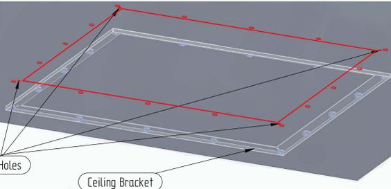
**Step 1** - Hold the ceiling bracket (the piece with the caged nuts) up to the ceiling, in the required mounting position and secure in place with 4 screws in the small corner holes then mark out the inner aperture (599 X 599mm +1/-1) and 16 bezel holes through the caged nuts. This installation is considered a two man operation.
