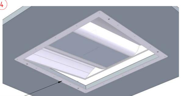
**Step 4** - Lift and tilt the 600x600 fitting into the void and then place on the holding bezel. Centralize the fitting (use fittings installation guide for instruction on this).
