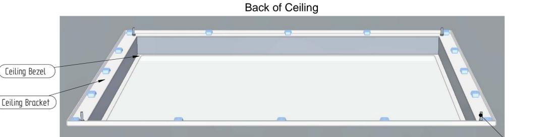
**Step 3** - Place the ceiling bracket into void and place it around the cut aperture. Then nut and bolt the ceiling bezel with dimples facing in the holes, these can be finger tight.
