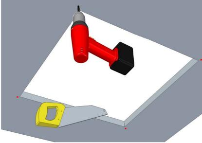
**Step 2** - Remove the ceiling bezel and 4 screws. Drill the 16 marked and 4 screw holes with a 10mm drill bit. Then cut the aperture for the fitting using the marked out lines. Ensure that the holes are drilled vertically as they need to align with the ceiling bracket cagenuts. (Cover kit will only work with 40mm Maximum Ceiling Thickness)
