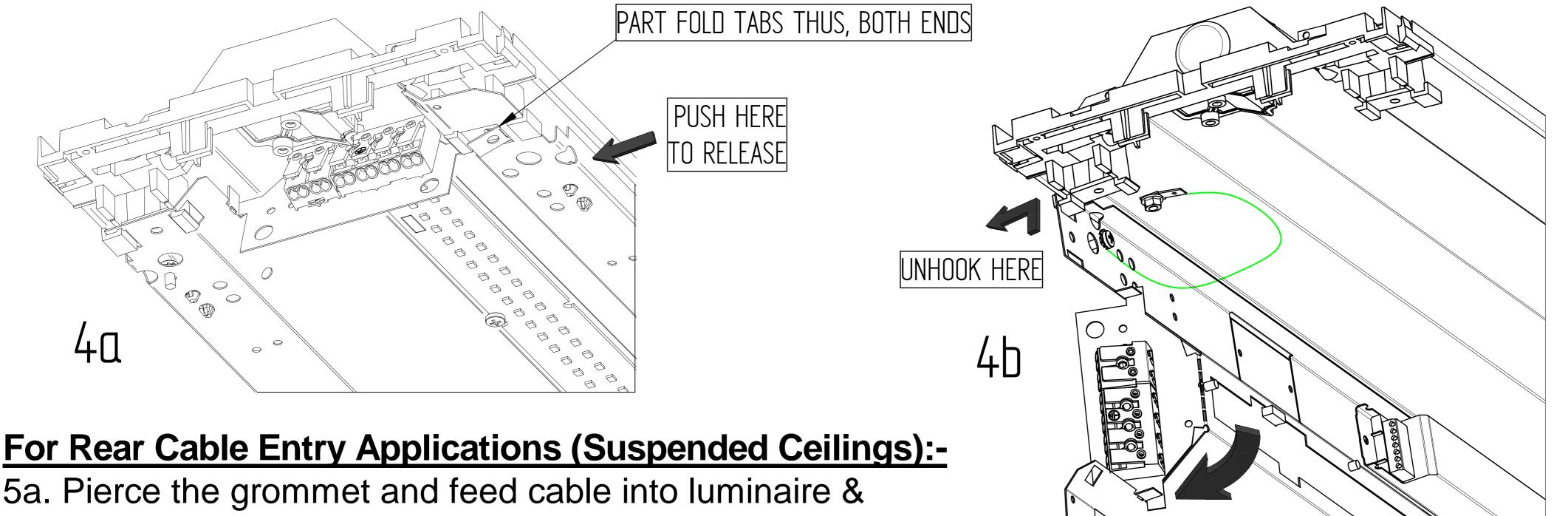
secure to the endcap using cable clamp & screws provided. Ensure there is 150mm of stripped cable available after the clamp. 5b. Fit the supplied sleeving over stripped cables between cable clamp & terminal blocks. 5c. Fix the canopy to the ceiling using appropriate fixings (supplied by others) via the 5mm mounting holes at centres indicated.
