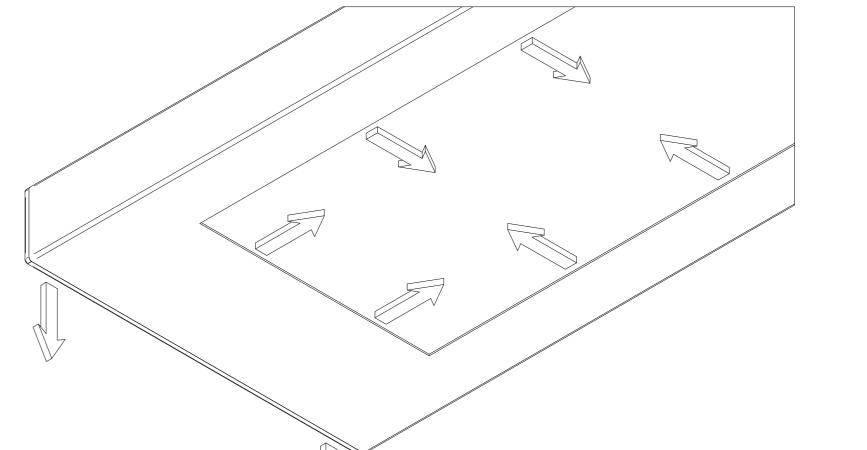
3. Remove the front diffuser optic assembly from the product by pushing up vertically & unhooking edges. Disconnect the safety & earth cords & sensor connection plug where fitted & set assy aside.
