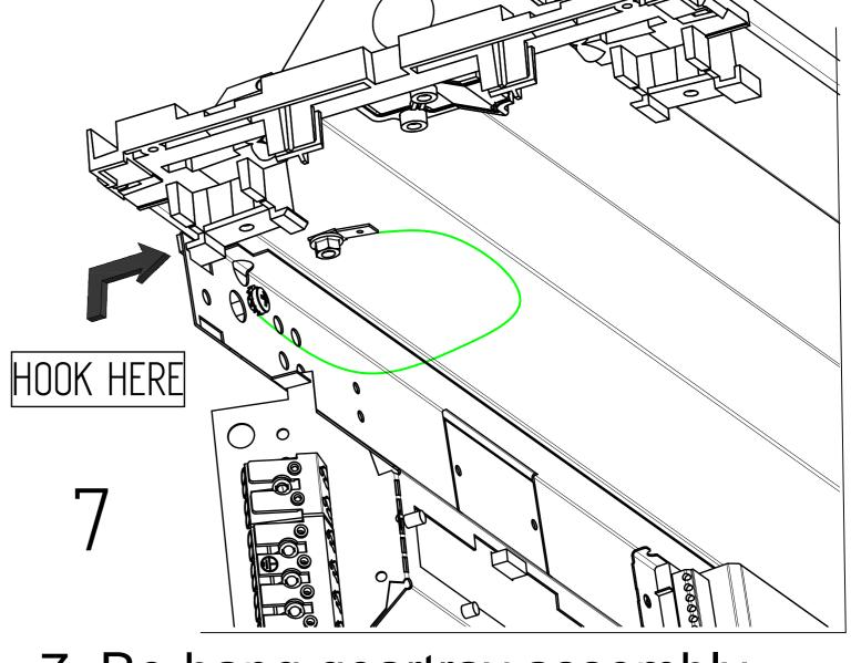
7. Re-hang geartray assembly onto the endcap clips at both ends & re-connect the earth lead.
