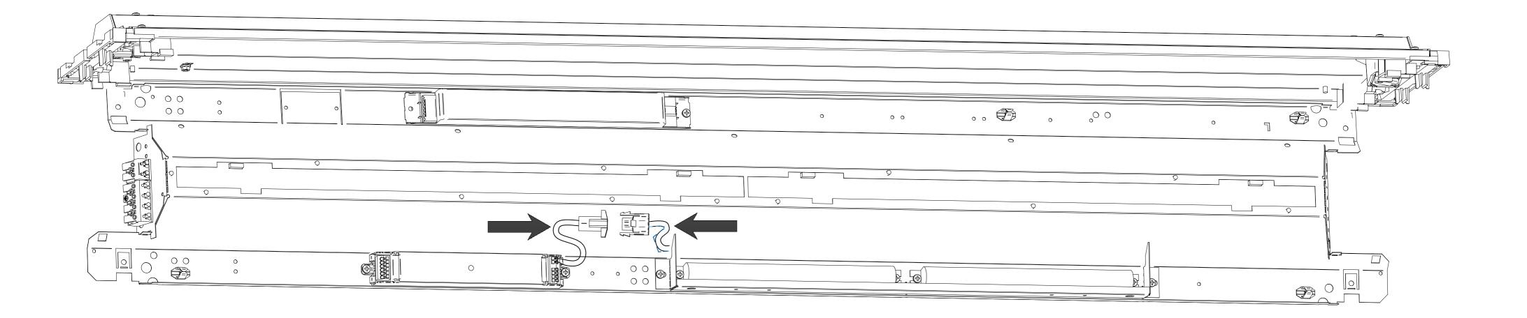
10. Refit the geartray assembly to the horizontal position ensuring that the plastic clips are fully engaged at both ends & the locking tabs are folded flat to their original position.
