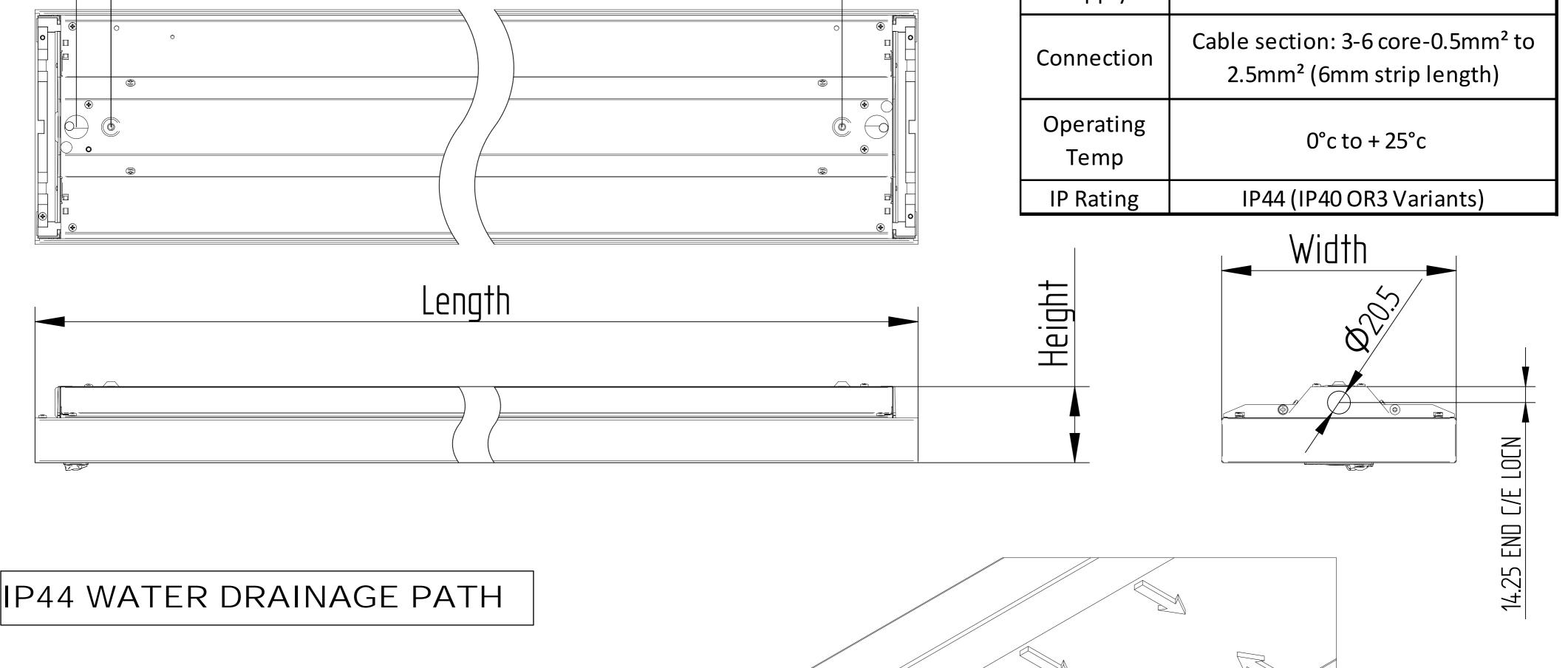
Drainage Path for any ingresss of water via diffuser & endcap joint as indicated right.
