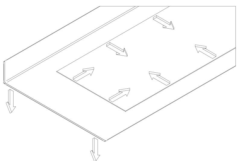
3. Remove the front diffuser optic assembly from the product by pushing up vertically & unhooking edges. Disconnect the safety & earth cords & sensor connection plug where fitted & set assy aside.
