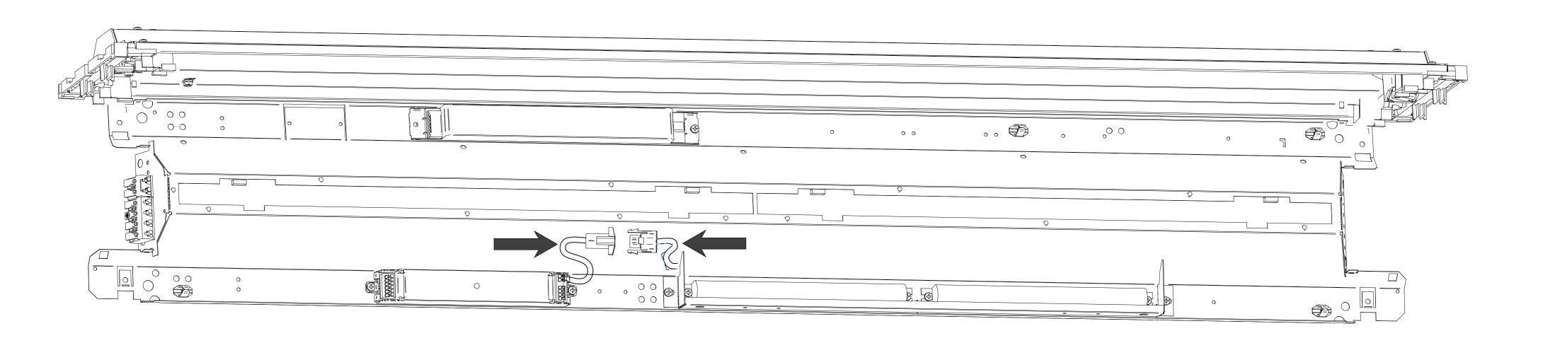
10. Refit the geartray assembly to the horizontal position ensuring that the plastic clips are fully engaged at both ends & the locking tabs are folded flat to their original position.
