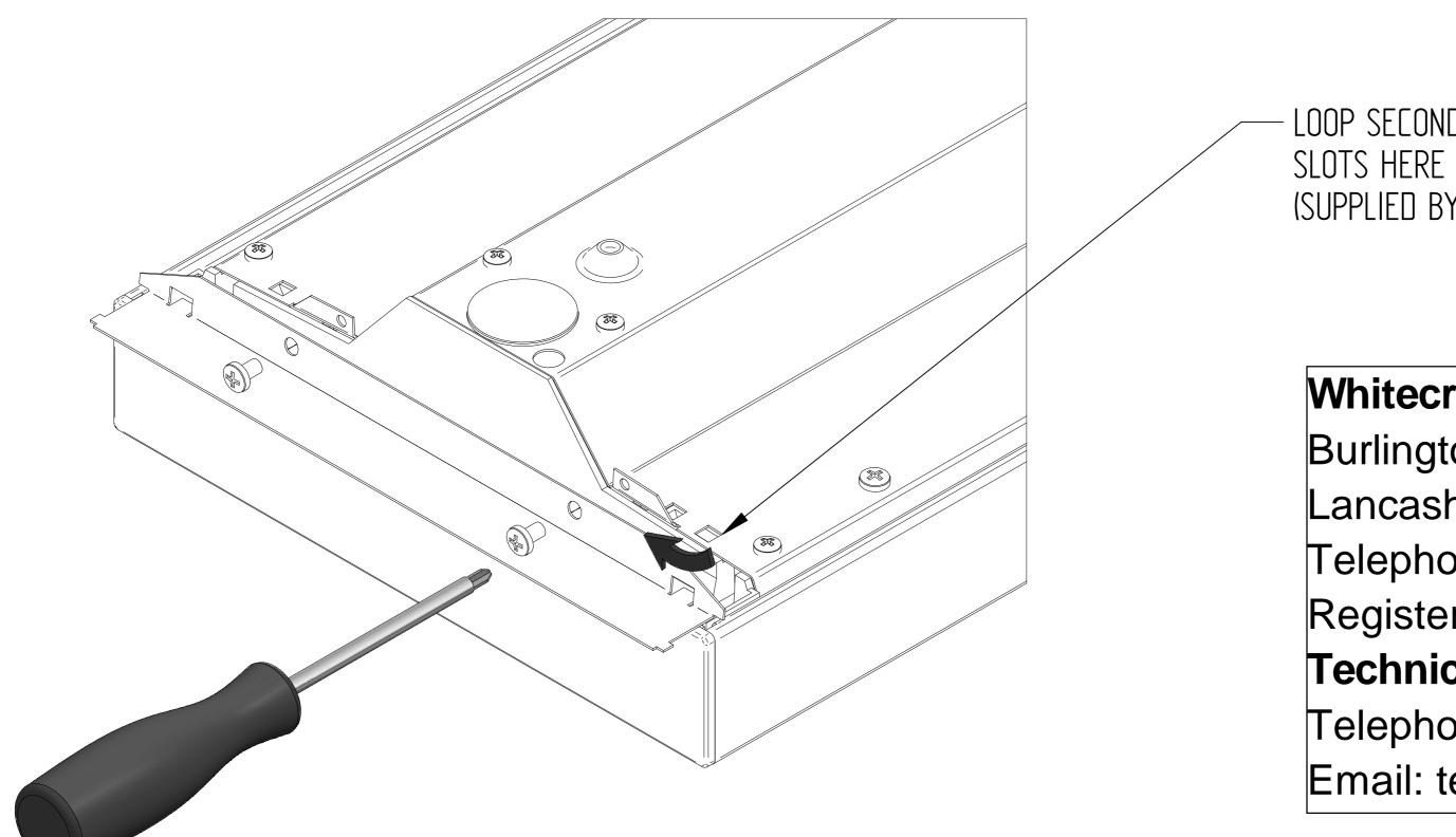
LOOP SECONDARY SUSPENSION CABLE THROUGH SLOTS HERE WHEN NECESSARY. (SUPPLIED BY OTHERS)
