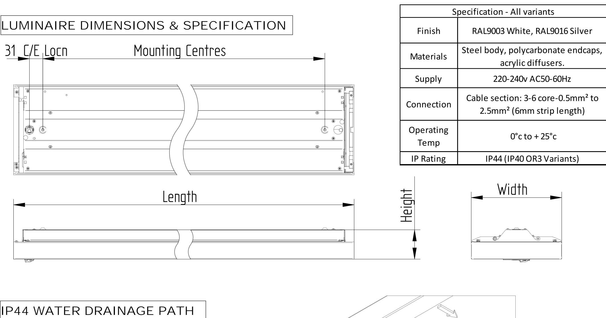
Drainage Path for any ingresss of water via diffuser & endcap joint as indicated right.
