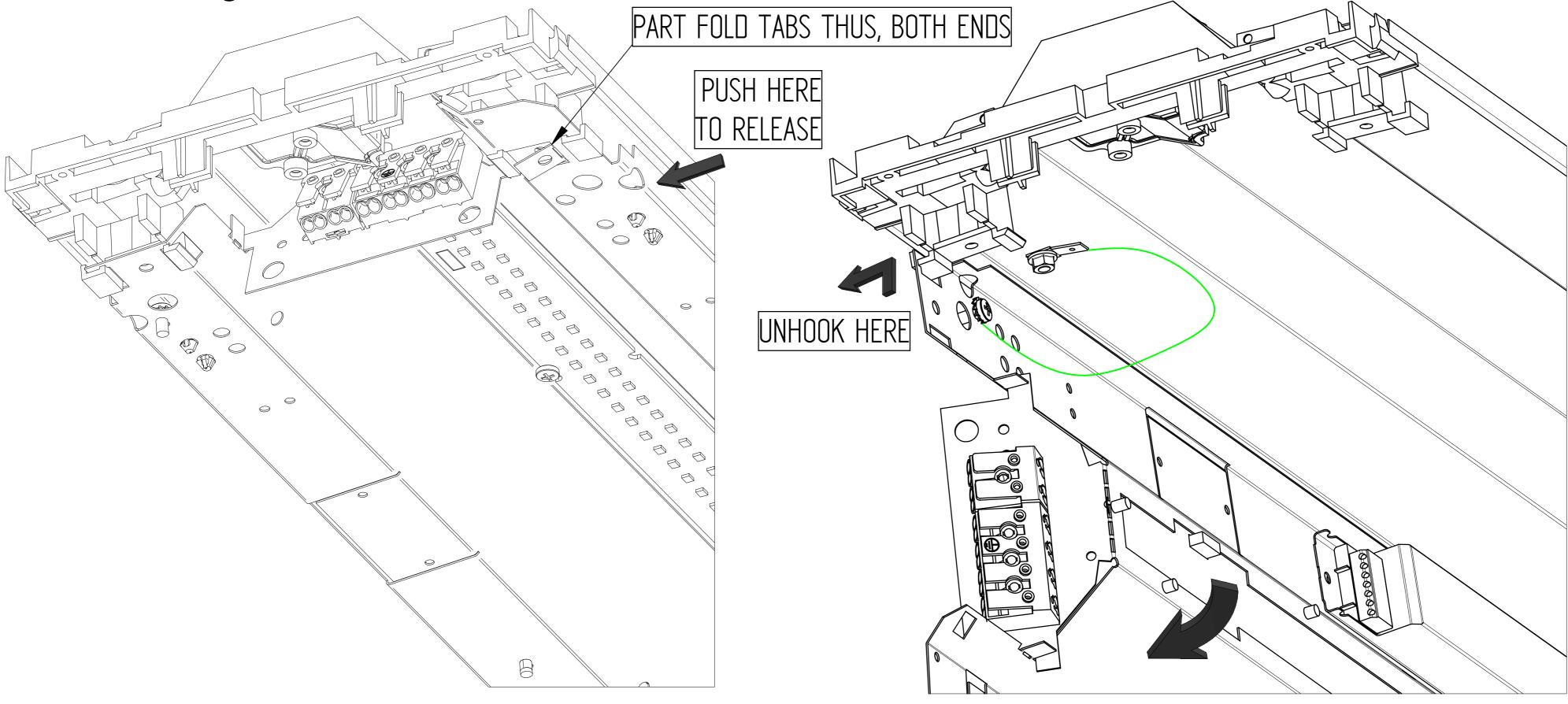
5a. Pierce the grommet and feed cable into luminaire before securing to endcap using clamp & screws provided. Ensure that there is 150mm of stripped cable available after the clamp. (See note re separate emergency Dali cable entry)
