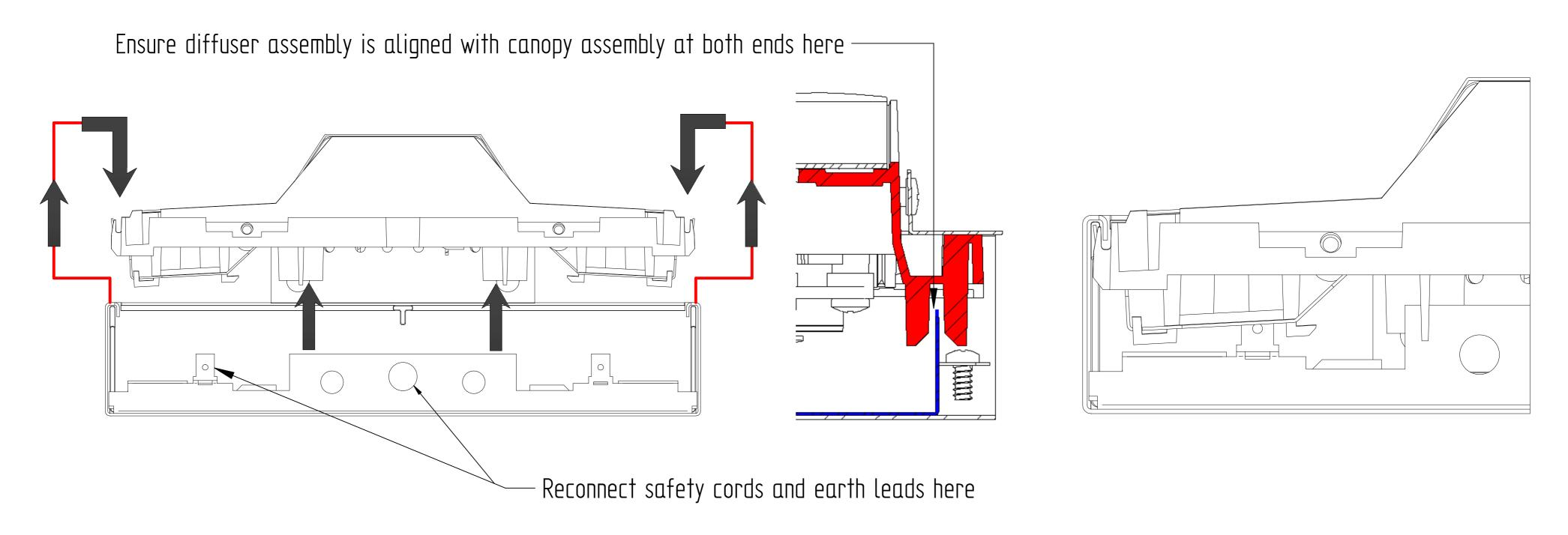
13. Fit locking plates at each end of luminaire with screws provided.
