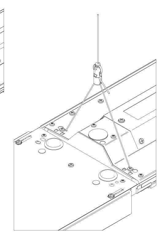
c)Fit the supplied jointing screws into the adjacent luminaires, but do not fully tighten at this stage.
