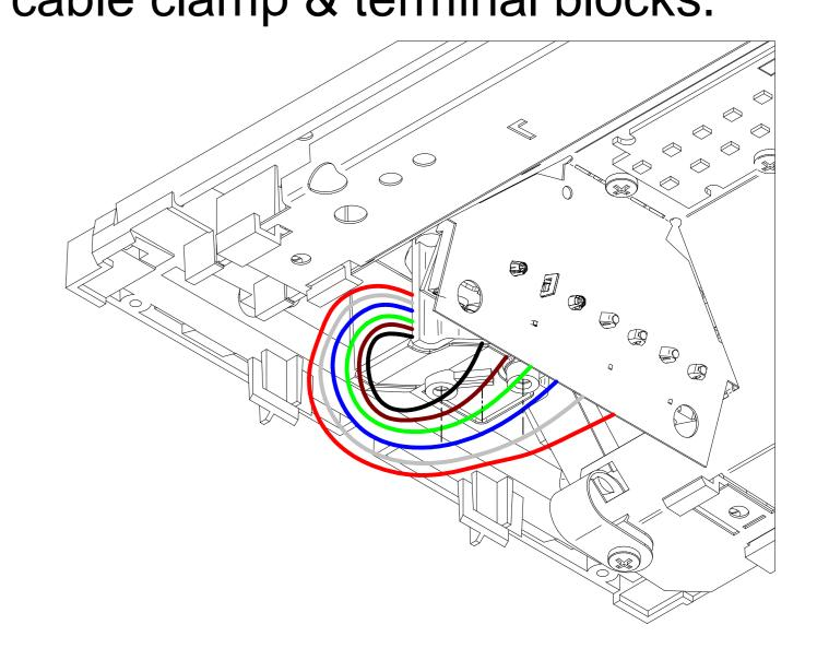
7. Wire mains / Dali cable into the Luminaire terminal blocks as per below (variant dependant)
