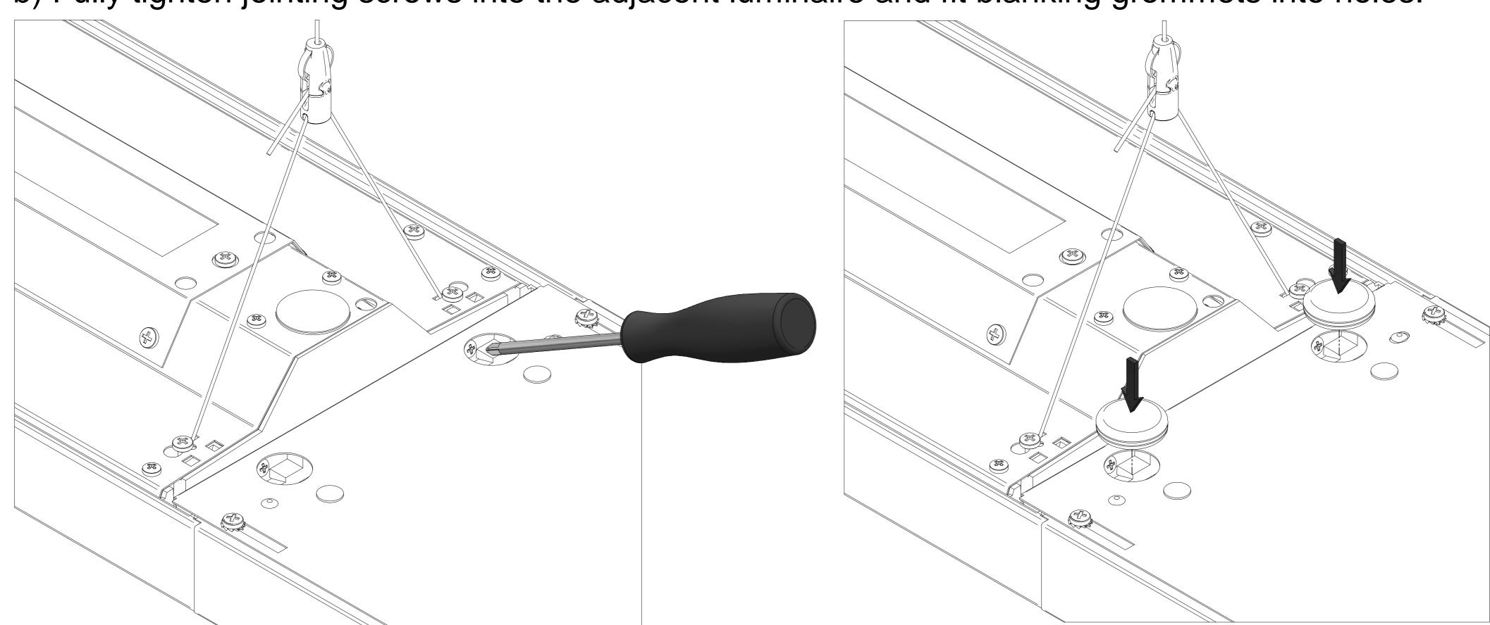
12. Fit locking plates at each end of continuous rows & individual luminaires with screws provided. Ensure that the plate overlaps the outer endcap at each end before fully tightening the screws.
