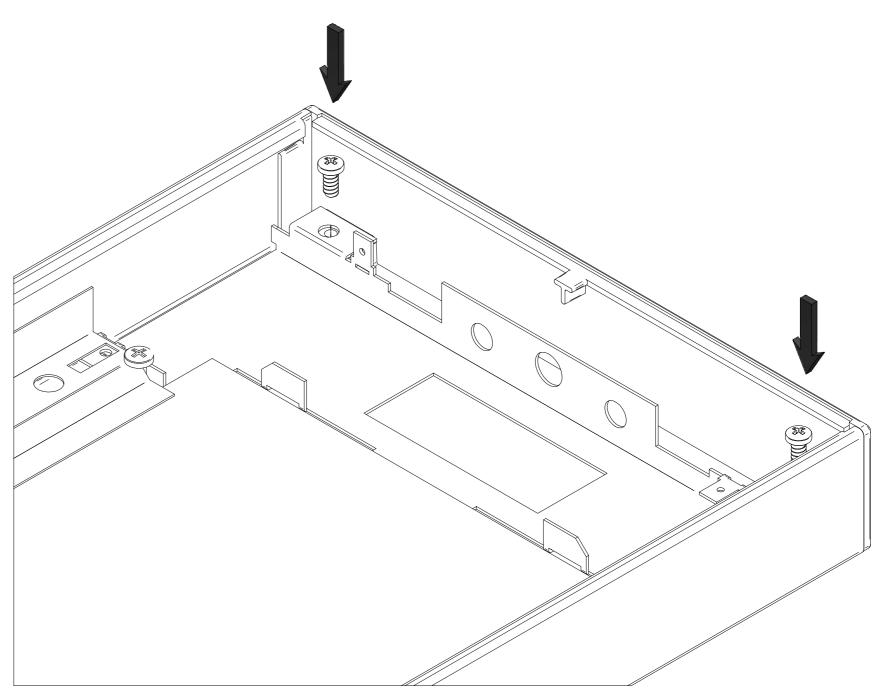
10a. Re-attach earth & safety cords to the diffuser assembly & connect Sensor plug where fitted. 10b. Align the front diffuser assembly with the canopy & re-attach to canopy by pushing up from the front until hook on both sides are fully clipped over the canopy edge along the entire length. Nb Care should be taken to ensure that no cables are trapped during the fitting process.
