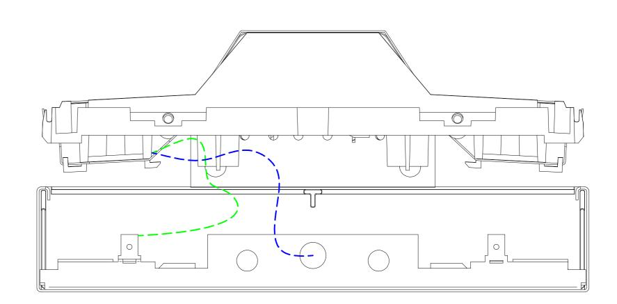
5a. Fit 'Y' splitter adjustable suspension hanger cables into the canopy keyhole cutouts and fit the included locking screws into the adjacent holes to secure.
