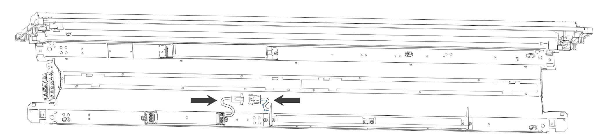
d) Refit the geartray assembly to the horizontal position ensuring that the clips are fully engaged at both ends & the locking tabs are folded flat to original position.
