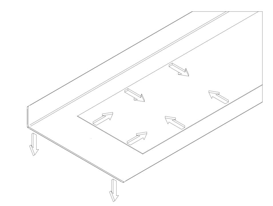
Drainage Path for any ingresss of water via diffuser & endcap joint as indicated above.
